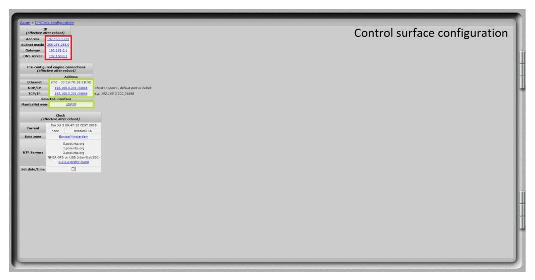
Then check at the Control surface configuration page if the Racks network IP adress, Subnet mask, Gateway and DNS server are correct (Shown in the red box). Off course the IP address should be different in the 4th block.
